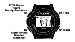
**Mode Control:** Press S4 button to change the Mode according to the following order:
